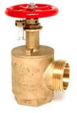
$2\frac{1}{2}$ " FxM combination angle hose and pressure restricting valve adjustable up to 300 lbs. Automatically drains and vents against hose deterioration. Locking pin device restricts full opening of valve. ULC, UL and FM Listed.
