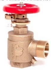
1½" FxF or FxM combination angle hose and pressure restricting valve adjustable up to 300 lbs. Automatically drains and vents against hose deterioration. Locking pin device restricts full opening of valve. ULC, UL and FM Listed.
