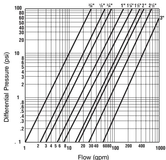
Flow curves show flows (gpm) and pressure drop (psig) using standard 20 mesh screen.
