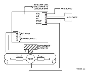
**NOTE:** WF input not required for keyswitch operation if waterflow detector is connected to panel or other monitoring device.
